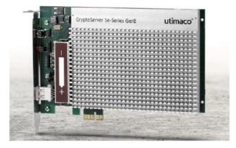
To enable communication of the cryptographic module with a host, the PCIe security module offers a PCIe interface and two USB interfaces. The PCIe security module is plugged into the PCIe bus interface of the backplane.
